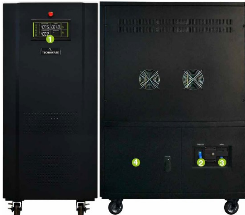
Figure 7 - Front side and left side FSTESC75KT - FSTESC100KT (1. Display, 2. Stabilizer Breaker, 3. Bypass Breaker, 4. Terminal Block Access Panel)
