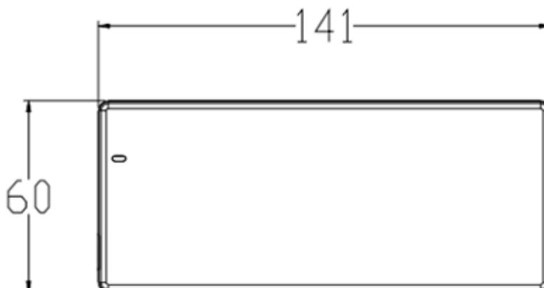
The model AP-FN90-24 charger by natural air. The input voltage range is 100-240Vac, the single-channel voltage is up to 29.2V, and the maximum current is 3A. The power supply has reverse polarity protection. The entire power supply is designed in strict accordance with safety regulations.
