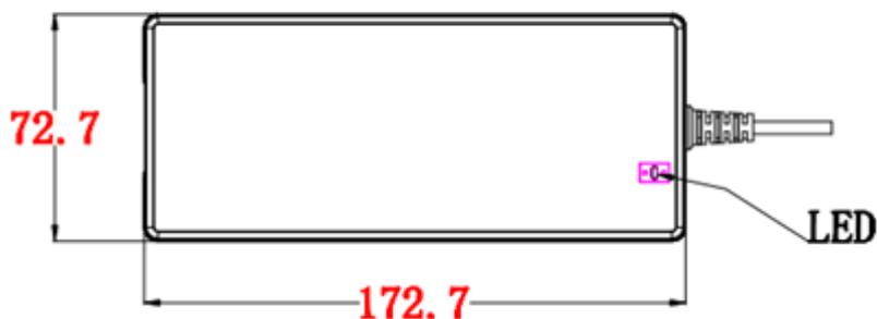
The model AP-PN120-12 charger by natural air. The input voltage range is 100-240Vac, the single-channel voltage is up to 14.4V, and the maximum current is 8A. The power supply has reverse polarity protection. The entire power supply is designed in strict accordance with safety regulations.
