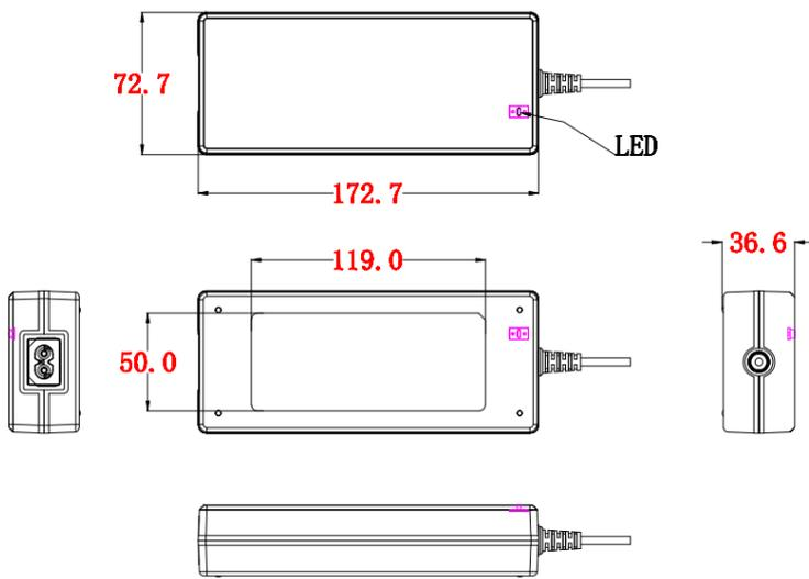
Tolerance of outline dimension is  $\pm 0.5\text{mm}$ , others are  $\pm 0.2\text{mm}$  in the diagram;
